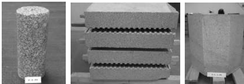
Fig. 2 The three types of laboratory samples: cylindrical (left), ctenoid (centre), and block (right).
