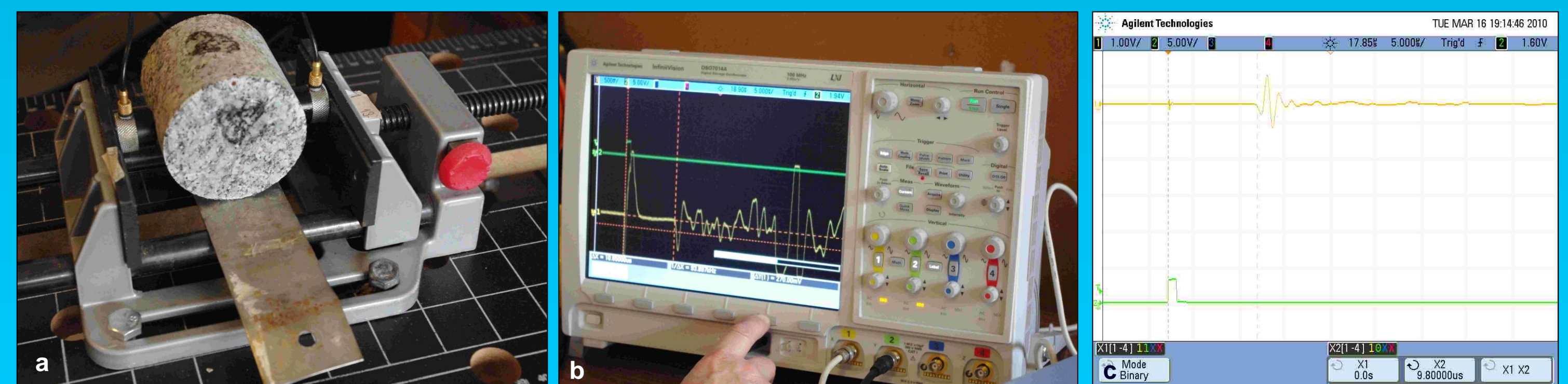
Fig. 2. a) Piezoelectric sensors on the granite core sample, b) oscilloscope during the measurement, c) record of P-wave
